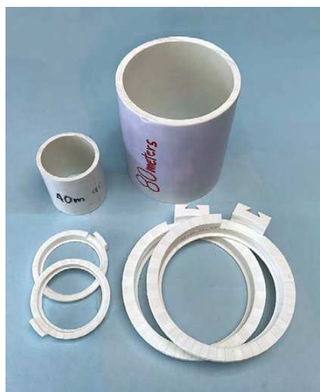
Figure 1 — End caps and body pipes. Note ramps on rings to keep turns together.
