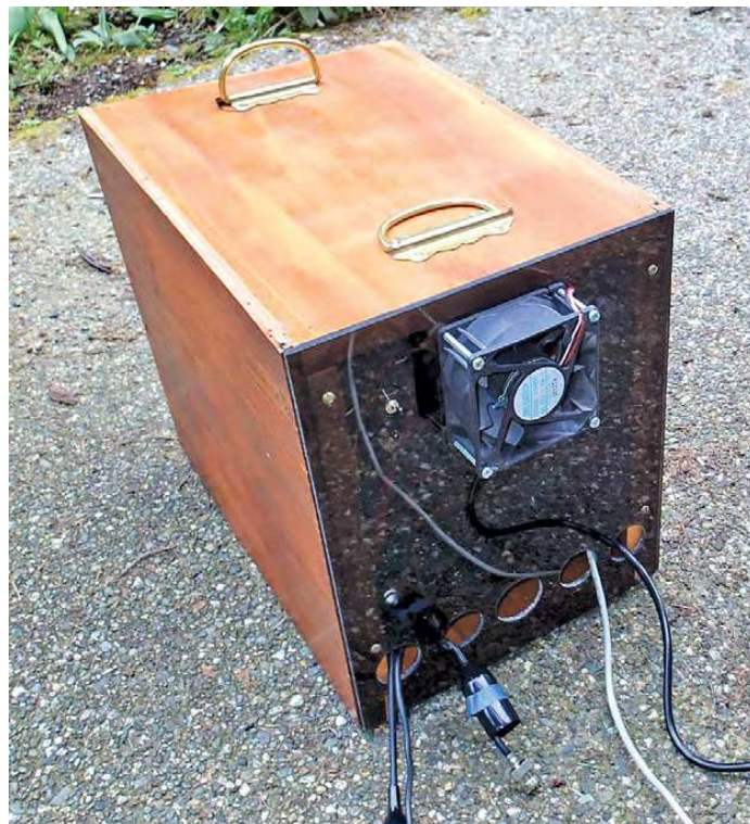
The completed station in a box with Plexiglas. Note the coax antenna plugs, ground wire, network, and power cables.
