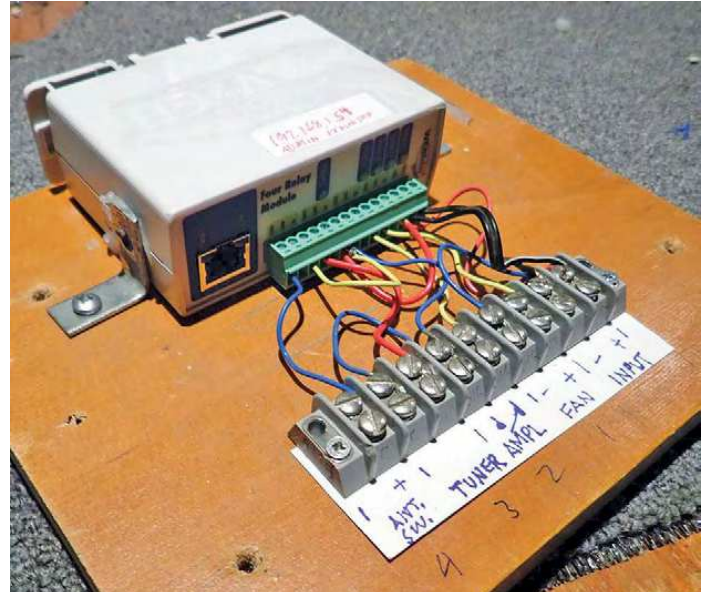
The web relay and terminal strip mounted to a scrap piece of wood for testing.
