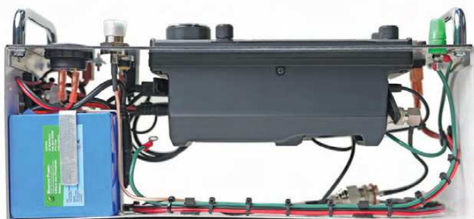
Figure 7 — Top view of the interior custom-built aluminum chassis of the IC-705 Go-Bag.
