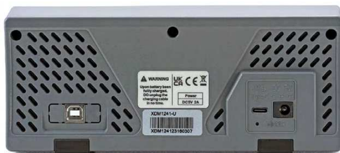
Figure 4 — The Owon XDM1241 rear panel has the 5 V dc power connector jack on the right; a similar model replaces this subassembly with a 120 V ac line voltage connector.
