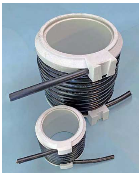
Figure 2 — Completed small 40-meter and large 80-meter un-ugly baluns.
