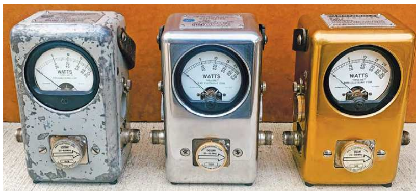
The Bird 43 wattmeter in three states: (left to right) the original, polished aluminum only, and with a translucent gold powder coat.
