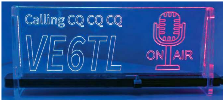
The ON AIR sign. The text on the right lights up when RF is detected.
