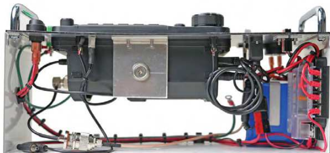
Figure 8 — Bottom view of the interior custom-built aluminum chassis of the IC-705 Go-Bag.
