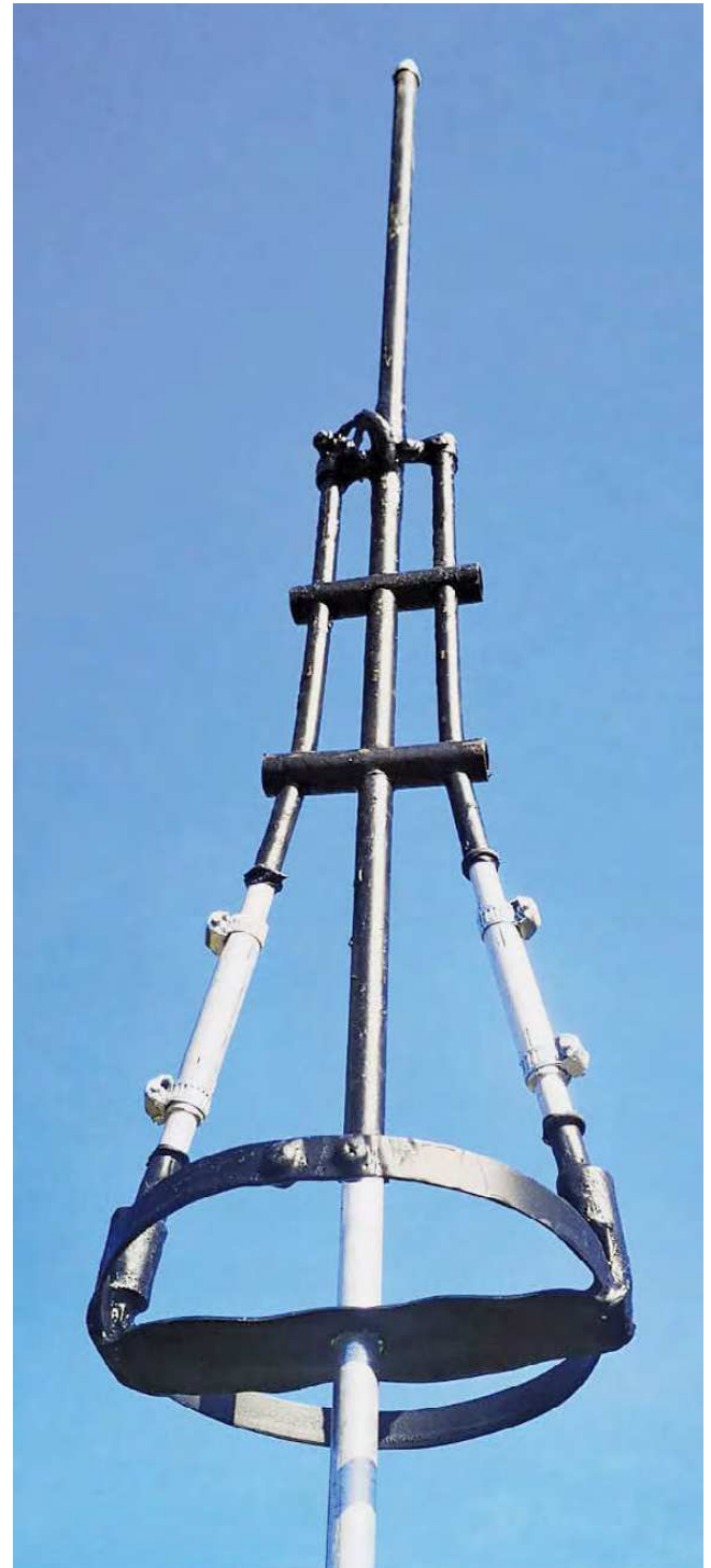
The Astroplane antenna modified for 2 meters.
