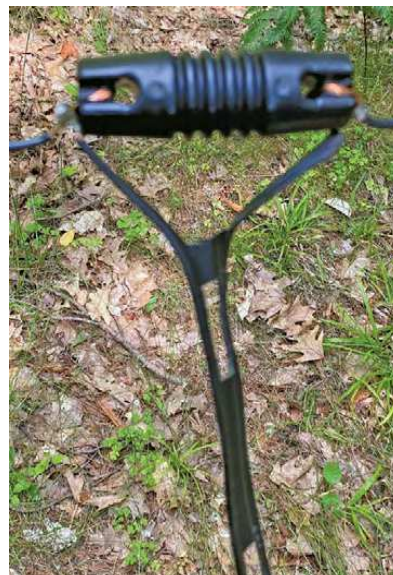
Figure 4 — Joining of wires to the ladder line.
