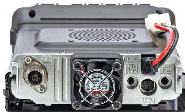
Figure 3 — The Yaesu FTM-500DR rear panel.
