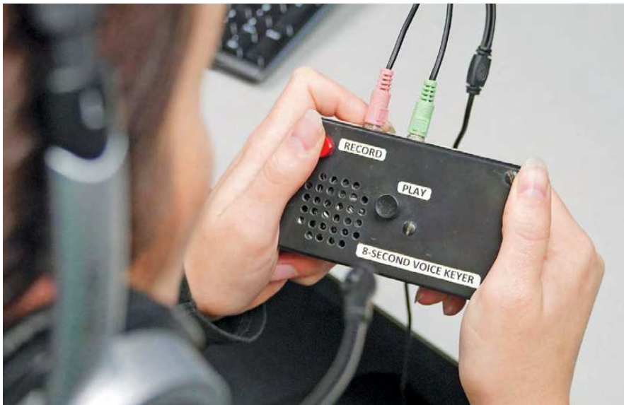
Figure 3 — Press and hold the red button on the top left corner of the keyer to record your 8- to 10-second message. Access the digital edition of QST ( www.arrl.org/qst ) to experience this voice keyer in action.
