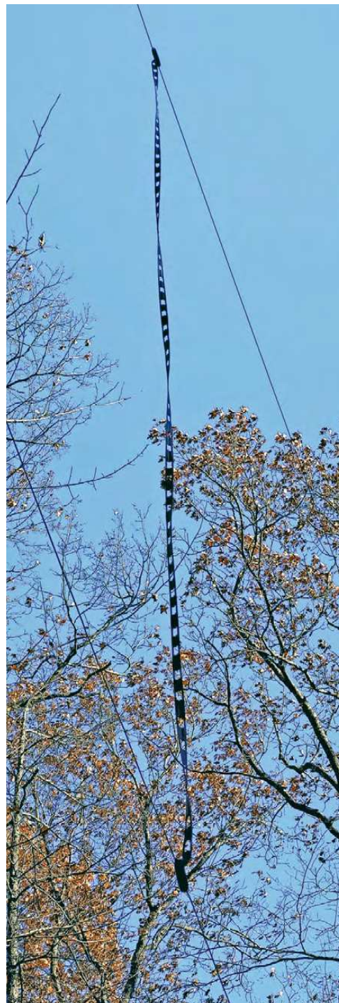
The antenna is difficult to see against the trees. The ladder line in this photograph seems to have several twists, but it has only one half twist.
