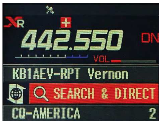
Figure 4 — The Yaesu FTM-500DR connected to the WIRES-X network repeater node.
