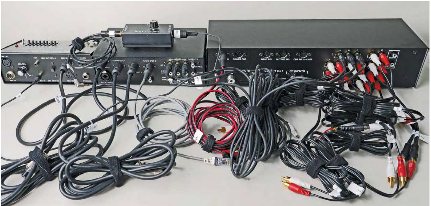
Figure 8 — The complete pre-wiring of all four pieces of W2IHY equipment.
