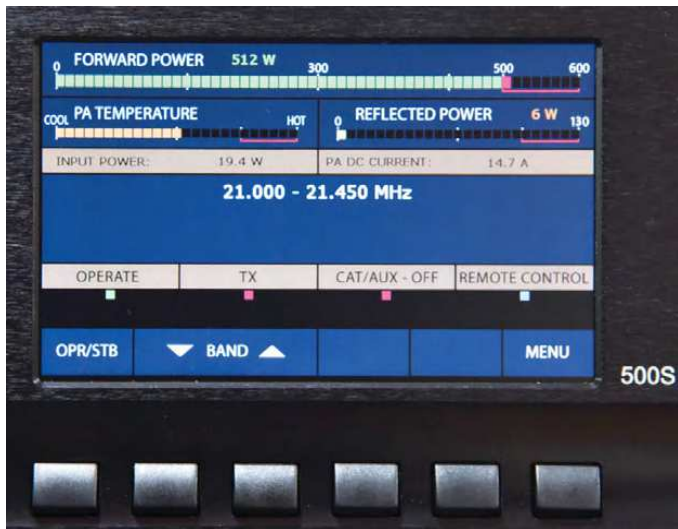
Figure 1 — The main operating screen shows important operating parameters such as selected band, forward and reflected power, drive power, and PA temperature. It's not a touchscreen — selections are made using the buttons below the screen. The MENU button at the lower right brings up various setup and monitoring screens.
