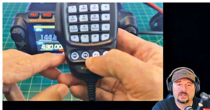
Ape walks viewers through the process of custom programming the microphone buttons on the Yaesu FTM-500D.
