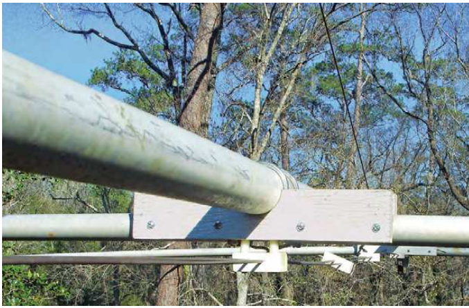
Figure 3 — The boom-to-element bracket with the feed-line spacer supported on standoffs. Just visible behind the spacer are the crossed wire jumpers from the antenna elements to the feed line.
