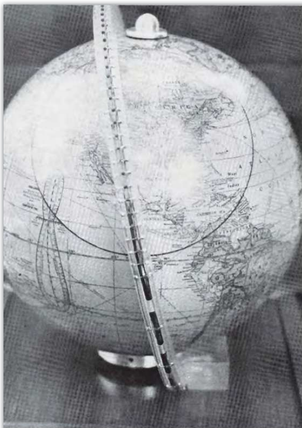
The Plexiglas ring has eyelets pressed into it to aid in making connections to the LEDs. The groove in the ring carries the wires from the LEDs to the base. A 2500-mile circle is shown centered on Salina, Kansas.
