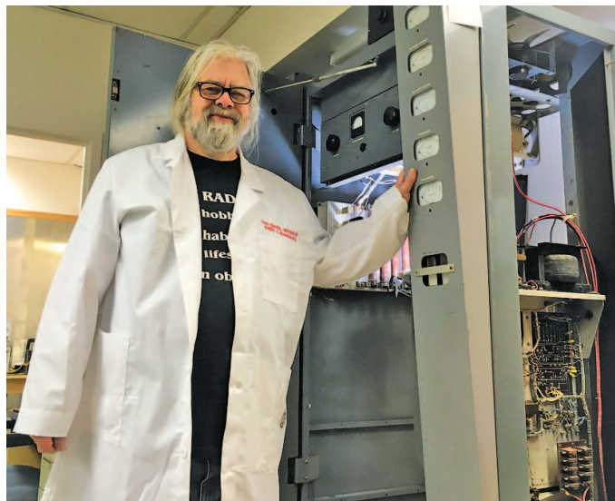
Tim "Timtron" Smith, WA1HLR, used his AM radio expertise to convert the BC-1T transmitter from broadcast to the ham bands.
