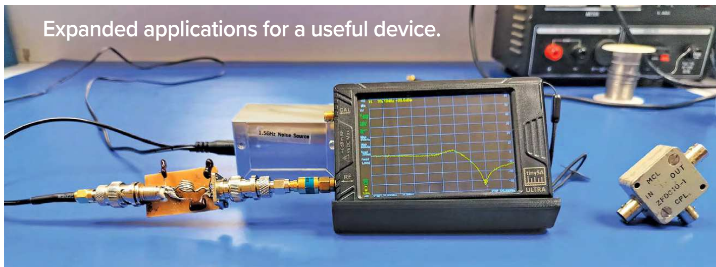
The 0.2 – 1500 MHz noise source and filter connected to the tinySA Ultra.
