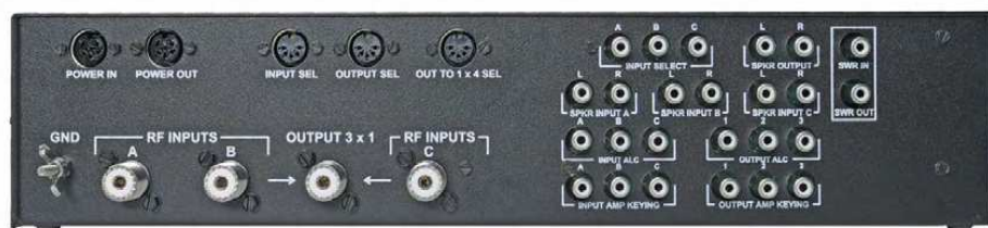
Figure 5 — The W2IHY 3 × 4 Switch Plus controller rear panel.
