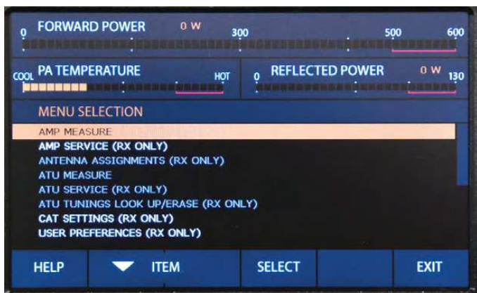
Figure 2 — The MENU screen is used to set up the amplifier. Several of the screen selections are not active without an ACOM automatic antenna tuner connected.
