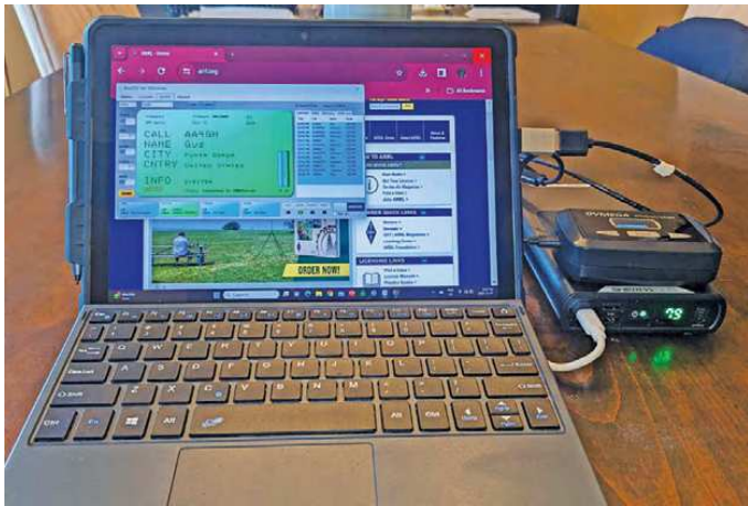
Figure 10 — The DVMEGA Globetrotter in AMBE dongle mode on the kitchen table.
