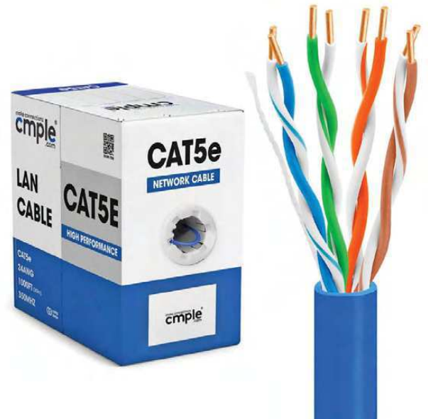
Figure 6 — Cat5e cable contains four pairs of color-coded wires, each with an accompanying white/color partner in a twisted pair. [ www.cmple.com ]
