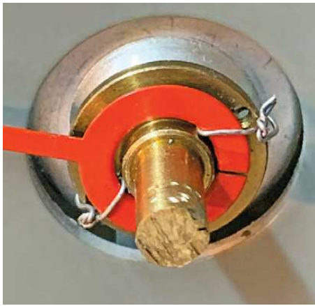
Figure 4 — The new vernier has two holes through which I threaded the wires and secured the pointer. [Dino Papas, KLØS, photo]
