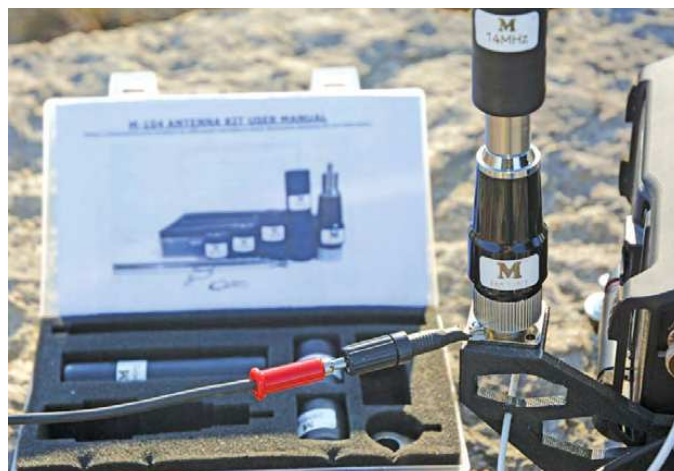
Figure 11 — A 3D-printed bracket with an SO-239 connector with the M-104 antenna. It works as expected on the Icom IC-705.
