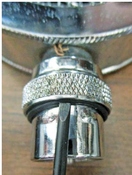
Figure 2 — A flat jeweler's screwdriver can be used to push the O-ring onto — and then behind — the threads of the knurled nut. [Robert W. Lobenstein, WA2AXZ/9, photo]
