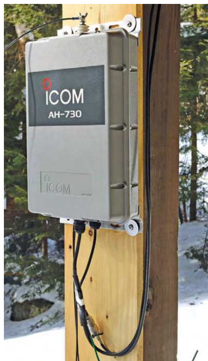
Figure 7 — An option is to mount the enclosure using wood screws or bolts and nuts. Here is the AH-730 attached to one of my deck supports and feeding an 85-foot end-fed wire.
