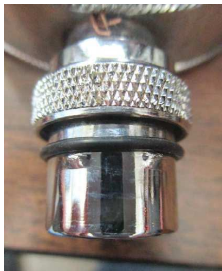
Figure 1 — The black O-ring in its initial position below the knurled nut, which is the collar portion of the microphone. [Robert W. Lobenstein, WA2AXZ/9, photo]
