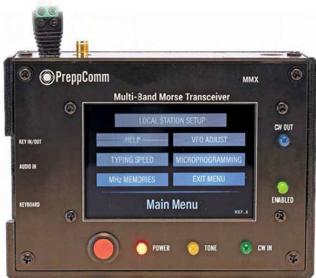
Figure 2 — The PreppComm MMX main menu has six choices, including the internal HELP system.
