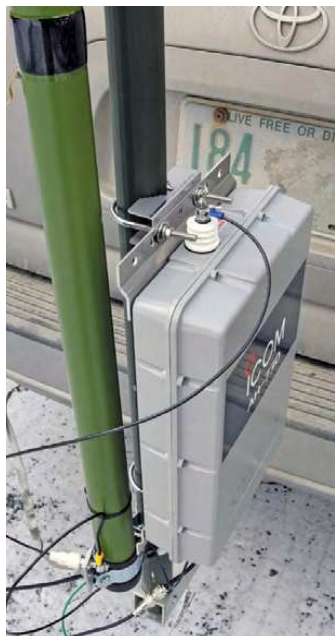
Figure 8 — The AH-730 package includes U-bolts for attaching the enclosure to a mast such as the support for the Eagle One vertical antenna on its trailer hitch mount.
