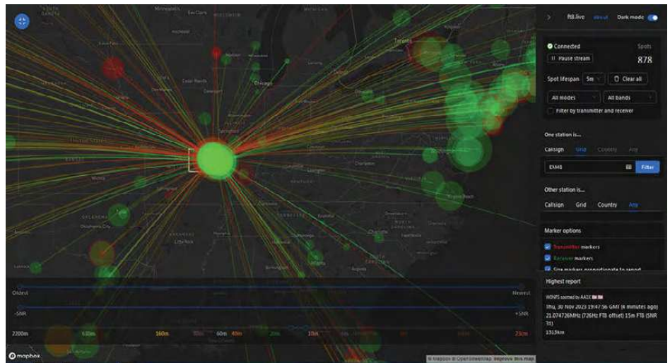
Figure 2 — FT8 Live map display (in optional dark mode) showing signals sent and heard in grid locator EM48 on the 15-meter band over the last 5 minutes. Note the sliders at the bottom of the map for controlling the age, SNR, and frequency band of the spots. [Ira Brodsky, KC9TC, photo]
