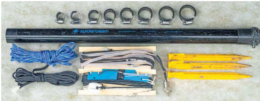
Figure 3 — The completed portable Zepp antenna prior to being deployed.
