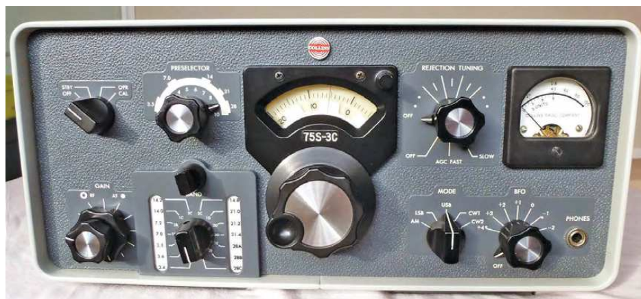
The Collins Radio 75S-3C used the same mechanical filters as the Hammarlund HQ-215. [Photo courtesy of www.radiopics.com ]
