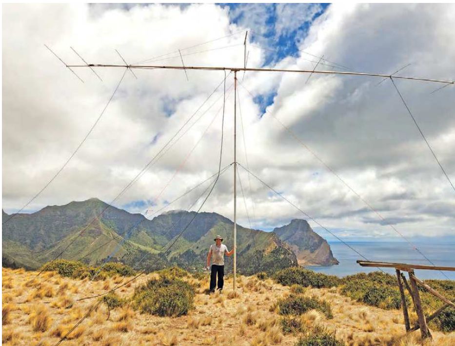
The CBØZA team's 6-meter M2 Antenna Systems 6M8GJ Yagi with Mike Crownover, Jr., AB5EB. [Mike Crownover, Jr., AB5EB, photo]
