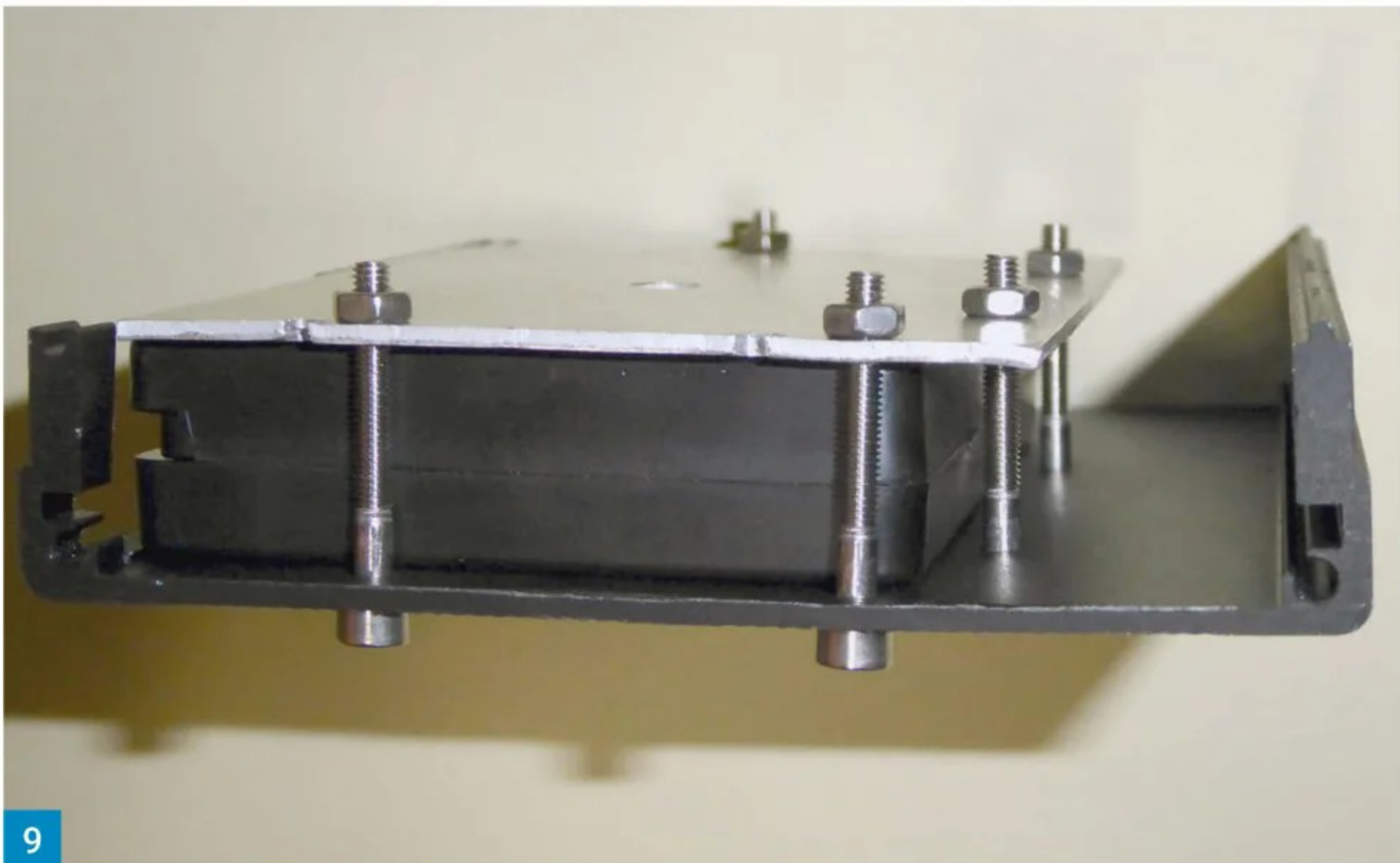
Fig. 8: Final retaining plate. Fig. 9: Retaining plate and VNA assembled to front panel. Fig. 10: Two halves ready to assemble. Fig. 11: Top controls. Fig. 12: NanoVNA with calibration pieces. Fig. 13: VNA in flight case. Fig. 14: Flight cases.
