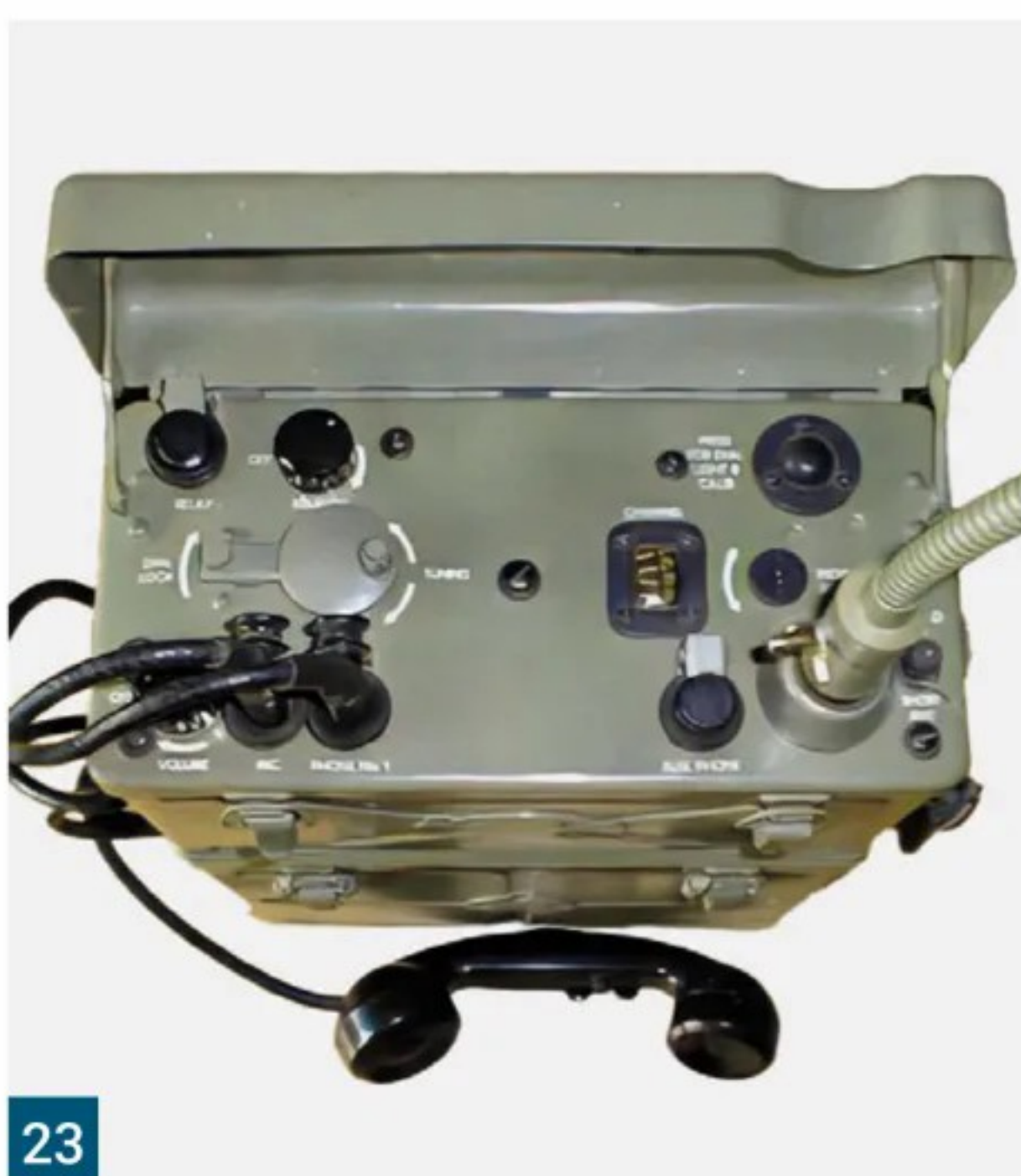
Fig. 18: The SCR-284 is a heavy AM set for communication between regiment and battalion and could not be operated on the move. In the field it was set up on extendable legs. The PE-104 vibrator powers the receiver when using the hand-cranked GN-45 generator. ( artstation.com ) Fig. 19: First introduced in 1942 for the invasion of North Africa, the SCR-284 saw service in the Pacific war and in NW Europe, when over 50,000 sets were allocated to US forces in June 1944 for D-Day. ( artstation.com ) Fig. 20: Merrill's Marauders in a clearing behind Japanese lines operating an SCR-284 radio. Note the mules in the background, which were used to transport the set in three separate 17kg loads. ( n6cc.com ) Fig. 21: This SCR-284 is being operated aboard an amphibious landing vessel. EIMAC Inc. produced radio power vacuum tubes (valves) and this was the cover picture of their news magazine for June 1945. ( n6cc.com ) Fig. 22: Nicknamed the true Walkie-Talkie, the SCR-300 launched in 1943. Galvin Inc. (today's Motorola) turned to the FM band as the solution for superior communication, range and portability, to create what is arguably the best portable radio of WWII. ( radiomilitari.com ) Fig. 23: A view of the SCR-300's top control panel and its HS-30 handset. ( wa8ywo.com ) Fig. 24: This control panel diagram is illustrated in the free online SCR-300 Technical Manual 1943 , found at repeater-builder.com/Motorola/pdfs/scr300.pdf Fig. 25: A US First Army signalman at a crossroads in Germany in 1945. The SCR-300 man-pack radio, with a range up to eight miles, was light enough to be operated by one man on the move.
