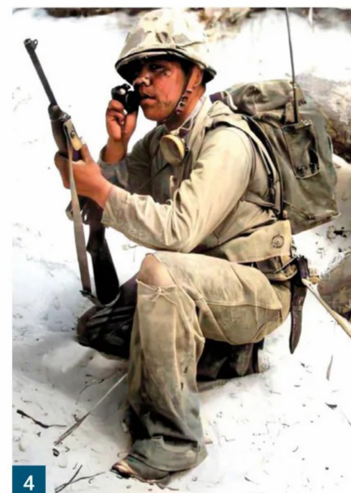
Fig. 1: TBV US Navy portable radios were used by the United States Marine Corps in the Pacific theatre, including by the Navajo Code Talkers speaking in their own unique language. Illustrated is the TBV-8 introduced in September 1943. ( usmilitariaforum.com ) Fig. 2: This lucky collector owns two TBV's, including their original canvas carry bags, antenna and headsets. Left: TBV-8 from September 1943. Right: TBV-2 introduced in January 1941. ( usmilitariaforum.com )
