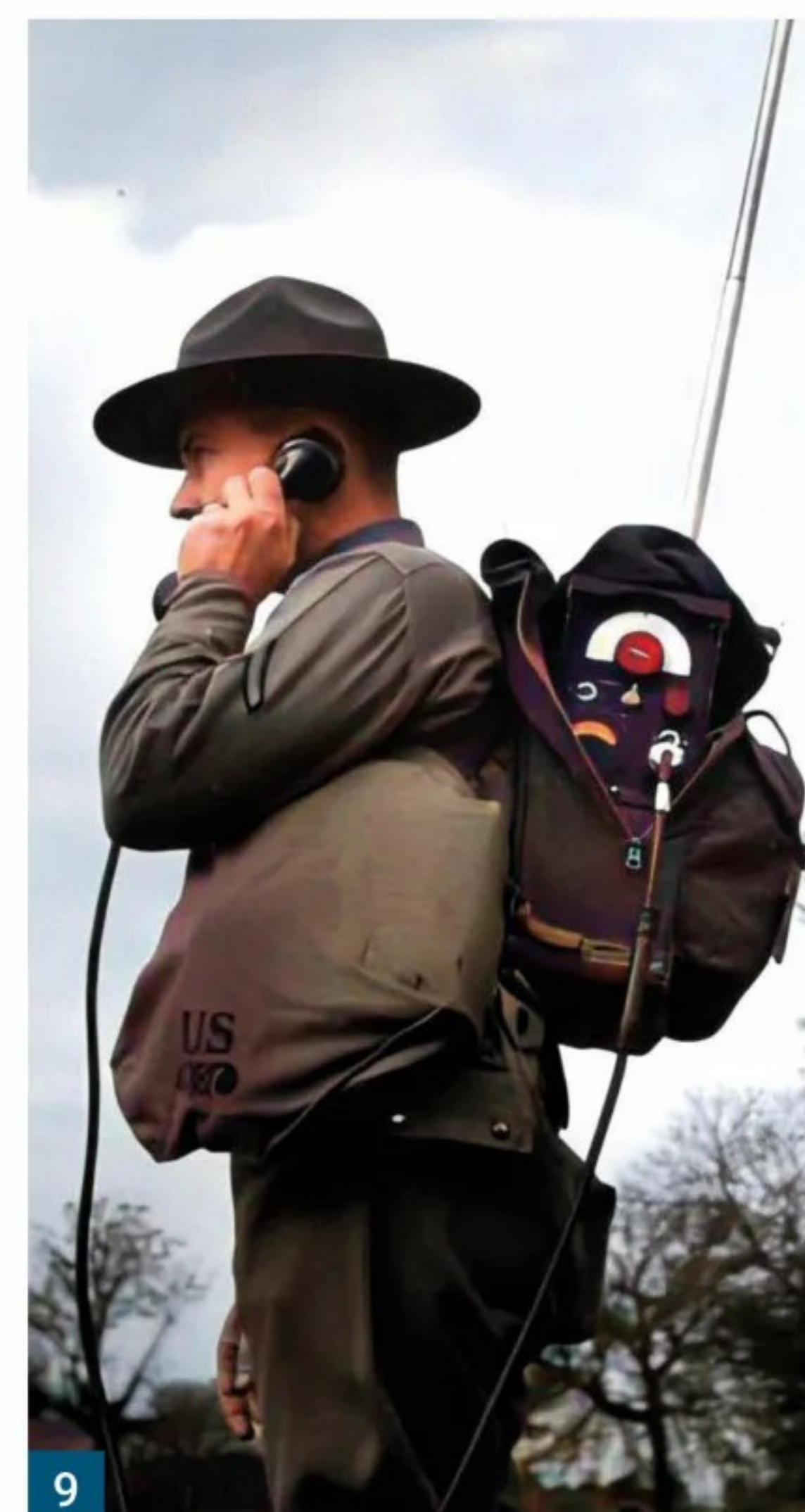
Fig. 3: The 30.7 x 30.1 x 18.4cm TBV's aluminium cabinet housed the transceiver and dry battery pack. Carried in a canvas case, together with the sectional antenna, the man-pack weighed 15.2kg. ( invaluable.com ) Fig. 4: A US Marine Navajo Code Talker operating his TBV radio. The Japanese were never able to understand their language, which proved to be more successful than using standard code. Fig. 5: The BC-322 transmitter-receiver for the lightweight SCR-195 radio is carried on the back of the operator in a canvas bag, together with the telescoping tubular antenna and battery, for a total weight of only 12.15kg. ( armyradio.ch ) Fig. 6: The lightweight SCR-195 portable company-battalion level radio, which had a range of up to five miles, is seen here inside its canvas backpack. ( imageevent.com ) Fig. 7: Left: the SCR-194 artillery observer version. Right: the SCR-195 infantry version. Also illustrated are the radio's backpacks, base for the antenna, TS-11 headset and box BX-13 for added connection ports. ( Radio-us-ww2.blog4ever.com ) Fig. 8: This pre-war publicity photograph illustrates the SCR-194 operated as a ground station. The operator is using a T-24 microphone and is wearing the TS-11 headset. ( timetoast.com ) Fig. 9: This photograph provides a clear understanding of how the lightweight SCR-195, when carried in a backpack, can be operated by one man on the move. ( life.com )
