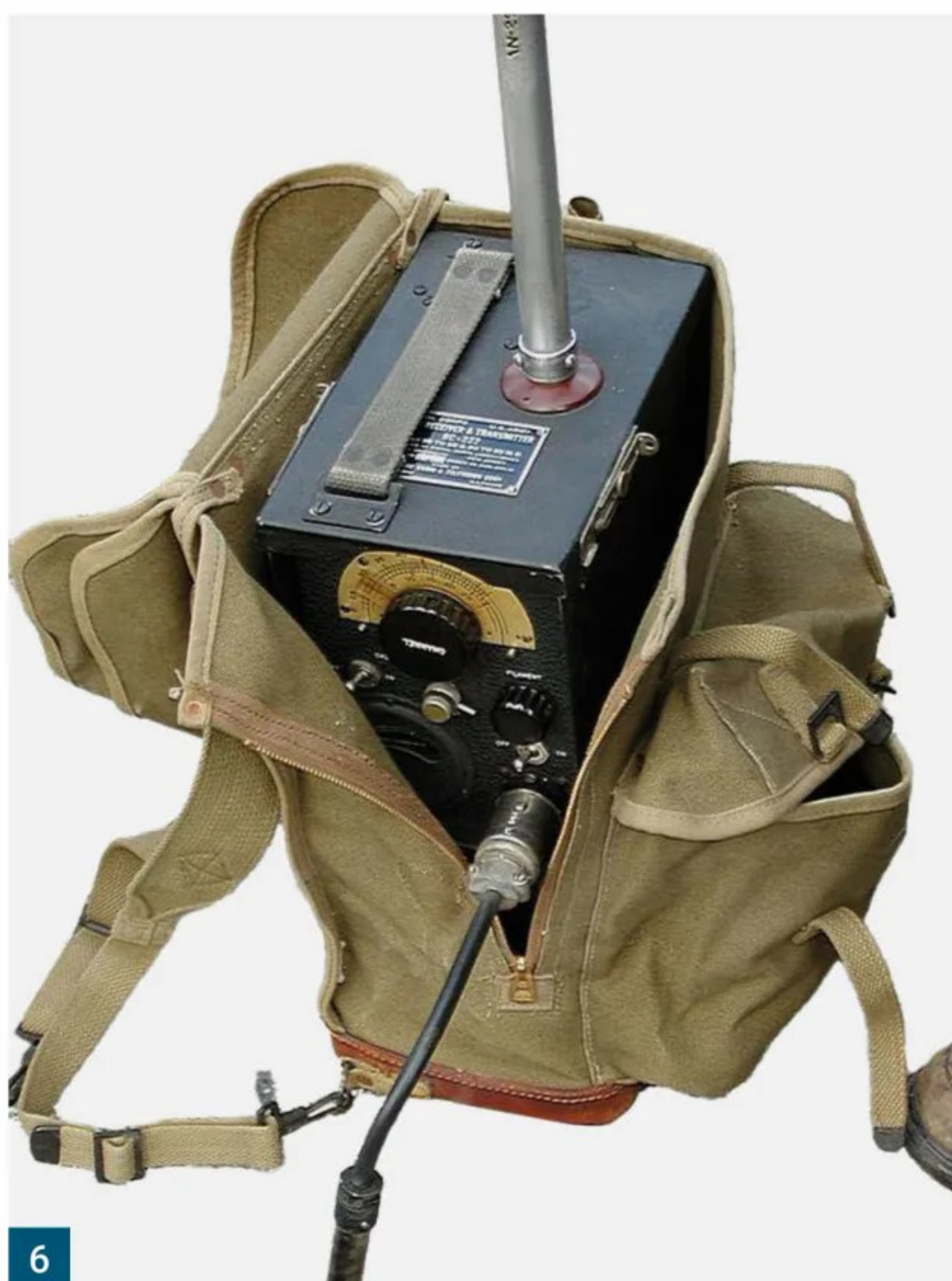
Fig. 1: TBV US Navy portable radios were used by the United States Marine Corps in the Pacific theatre, including by the Navajo Code Talkers speaking in their own unique language. Illustrated is the TBV-8 introduced in September 1943. ( usmilitariaforum.com ) Fig. 2: This lucky collector owns two TBV's, including their original canvas carry bags, antenna and headsets. Left: TBV-8 from September 1943. Right: TBV-2 introduced in January 1941. ( usmilitariaforum.com )
