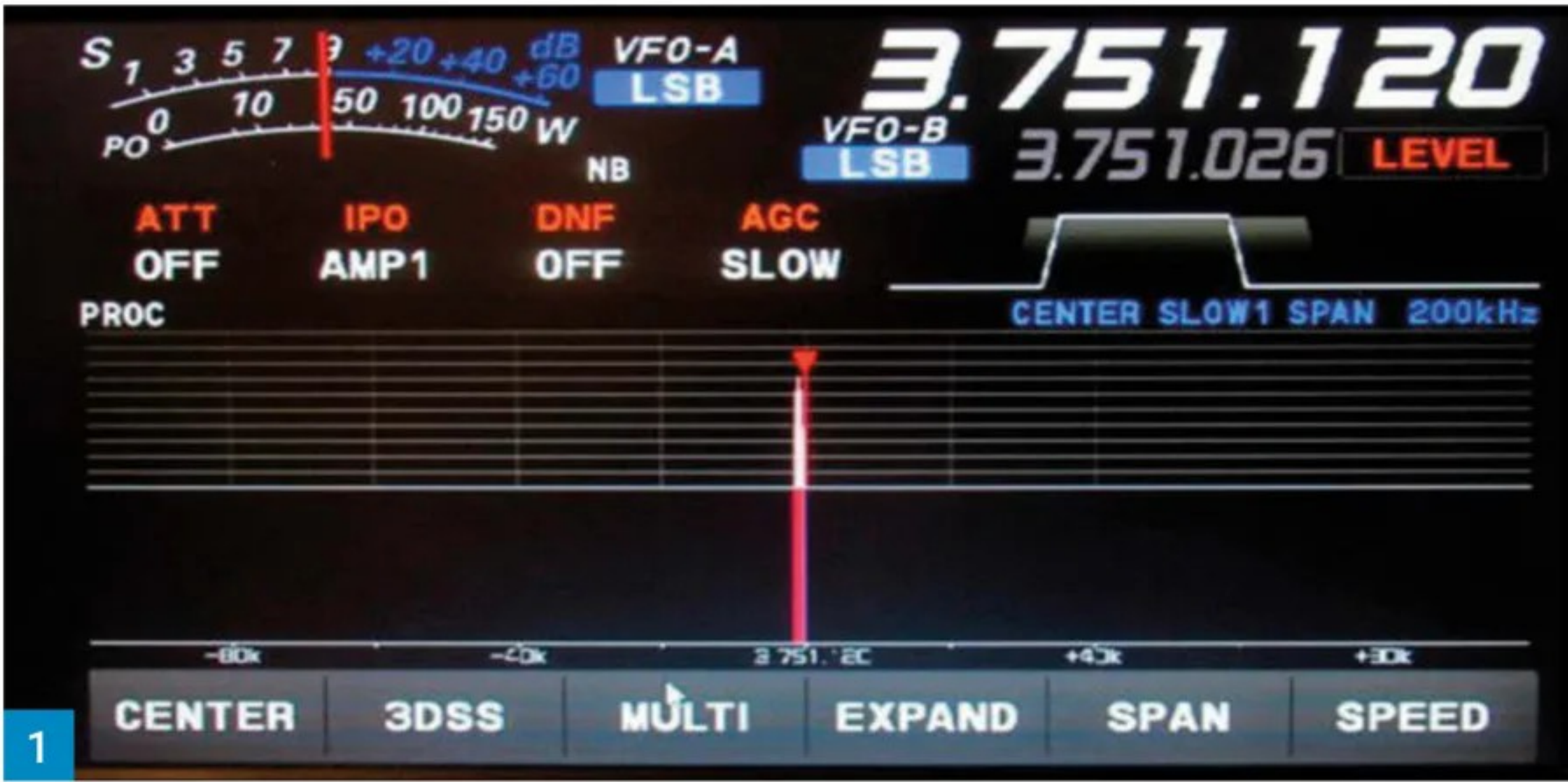
Fig 1: -73dBm signal, Amp 1, Vert. scale -110 to -60dBm, meter at S9, scope close to -73dBm. Level control set to 0dB. Level.
