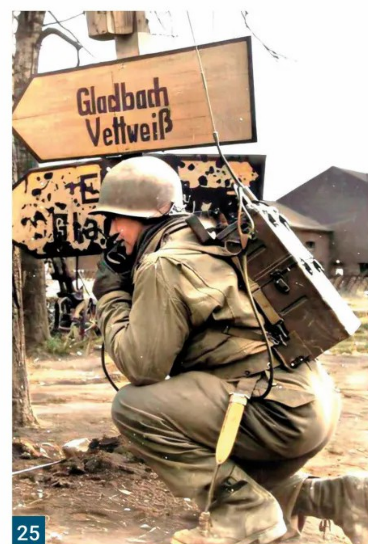
Fig. 18: The SCR-284 is a heavy AM set for communication between regiment and battalion and could not be operated on the move. In the field it was set up on extendable legs. The PE-104 vibrator powers the receiver when using the hand-cranked GN-45 generator. ( artstation.com ) Fig. 19: First introduced in 1942 for the invasion of North Africa, the SCR-284 saw service in the Pacific war and in NW Europe, when over 50,000 sets were allocated to US forces in June 1944 for D-Day. ( artstation.com ) Fig. 20: Merrill's Marauders in a clearing behind Japanese lines operating an SCR-284 radio. Note the mules in the background, which were used to transport the set in three separate 17kg loads. ( n6cc.com ) Fig. 21: This SCR-284 is being operated aboard an amphibious landing vessel. EIMAC Inc. produced radio power vacuum tubes (valves) and this was the cover picture of their news magazine for June 1945. ( n6cc.com ) Fig. 22: Nicknamed the true Walkie-Talkie, the SCR-300 launched in 1943. Galvin Inc. (today's Motorola) turned to the FM band as the solution for superior communication, range and portability, to create what is arguably the best portable radio of WWII. ( radiomilitari.com ) Fig. 23: A view of the SCR-300's top control panel and its HS-30 handset. ( wa8ywo.com ) Fig. 24: This control panel diagram is illustrated in the free online SCR-300 Technical Manual 1943 , found at repeater-builder.com/Motorola/pdfs/scr300.pdf Fig. 25: A US First Army signalman at a crossroads in Germany in 1945. The SCR-300 man-pack radio, with a range up to eight miles, was light enough to be operated by one man on the move.
